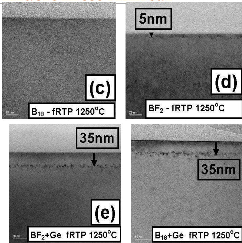
With diffusionless anneal, no EOR defects with  $B_{18}H_{22}$ .
