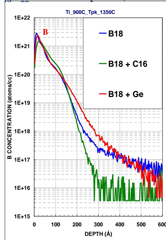
High boron concentration at Ge EOR defect region. Reduced concentration with C<sub>16</sub>H<sub>10</sub> at iRTP 900°C. The concentration is removed at the higher flash temperature Tpk = 1350°C.
