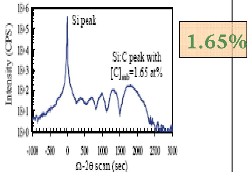
Fig. 2 HRXRD rocking curve of the SPE Si:C film ( $[C]_{sub}=1.65$  at%) grown on (100) Si substrate. The well defined Si:C peak and fringes indicate that the Si:C film is high-quality single crystal.
