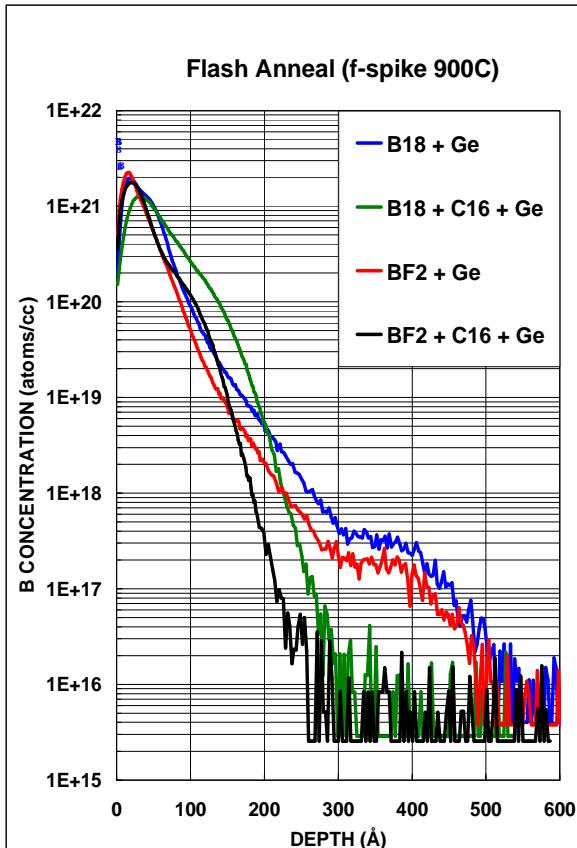
The pile up due to Ge implants is eliminated with C<sub>16</sub> co-implant
