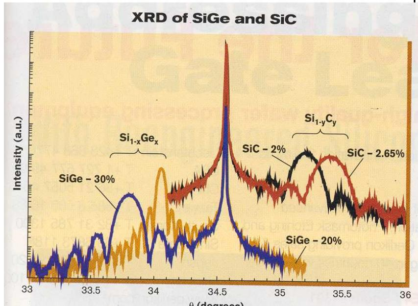
6. Different concentrations of  $\text{Si}_{1-x}\text{Ge}_x$  and  $\text{Si}_{1-y}\text{C}_y$  epi films used as pMOS and nMOS S/D stressors, respectively. Interference fringes indicate high crystalline quality.
