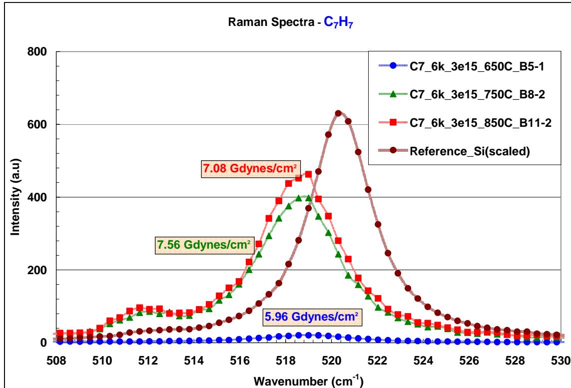
Strained layer thickness equal to the amorphous layer thickness for 750°C sample
