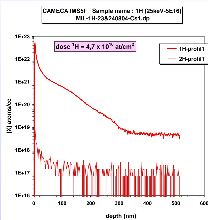
SIMS profile of Hydrogen implantation ( $5 \text{ e}^{16} \text{ cm}^{-2}$  - 25 kV)
