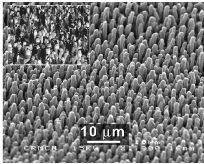
SEM photo of penguin-like structures created by femtosecond laser (top left corner is a picture of a real penguin colony in Antarctica, photo by G. DARGAUD [www.gdargaud.net](http://www.gdargaud.net)) (with courtesy of LP3)
