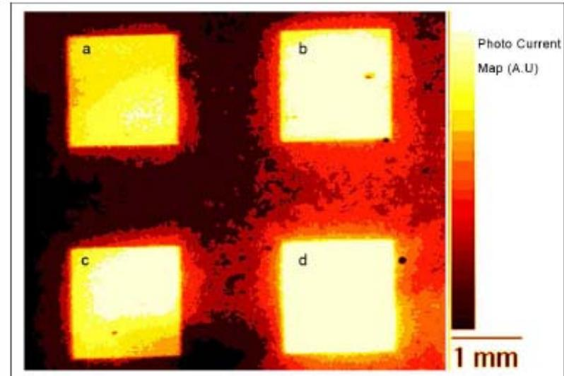
LBIC scan maps showing the increase of the photocurrent in the laser treated zones.
