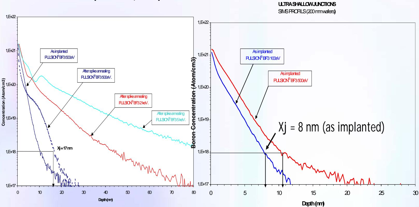
Exemple of BF3 PULSION® implantations from 100V to 5kV for USJ (IBS / LETI collaboration)
