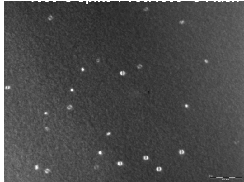
TEM WBDF image g=[422] after 1000 °C spike + 1300 °C flash
