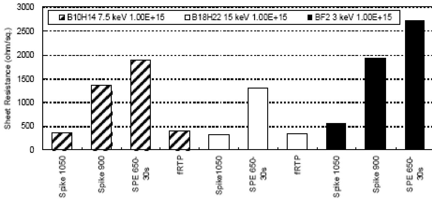
Fig. 3: Boron Rs for pSDE implants and anneals.
