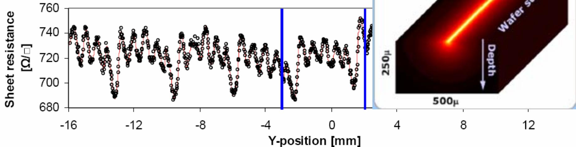
Figure 2: 30 mm sheet resistance line scan perpendicular to the laser scan direction using a 10  $\mu\text{m}$  pitch four-point probe and a step size of 25  $\mu\text{m}$ . The vertical lines define the area which was consecutively probed with different probe pitches (cf. figure 3). A continuous function of the sheet resistance was approximated (thin line) for finite element method (FEM),
