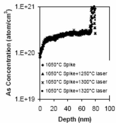
Arsenic SIMS-profiles in poly-Si with different laser annealing temperatures.
