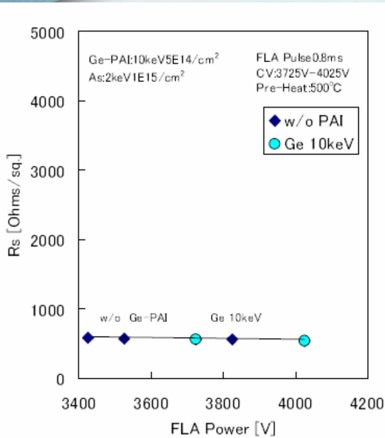
Fig.6 The dependence of lamp power in FLA on Rs of As doped n+/p junction
