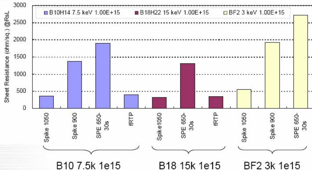
The larger B cluster size ion implantation obtained lower sheet resistance at SPER
