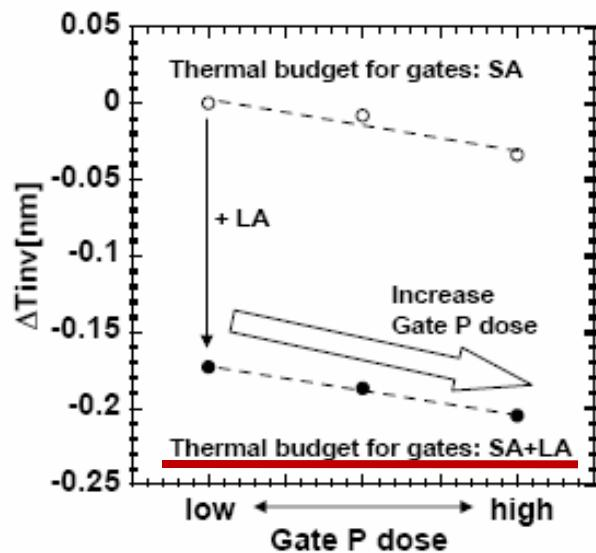
Fig.10  $T_{inv}$  (EOT + inversion layer + gate depletion) reduction with gate-poly pre-dope optimization for different thermal budgets (spike anneal (SA) or laser anneal (LA)).
