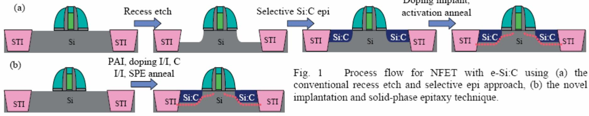
Fig. 1 Process flow for NFET with e-Si:C using (a) the conventional recess etch and selective epi approach, (b) the novel implantation and solid-phase epitaxy technique.
