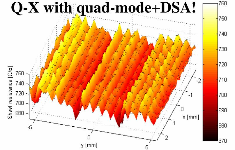
Figure 6: 45×101 point area scan measured with a 10  $\mu\text{m}$  pitch M4PP. The scan step size is 50  $\mu\text{m}$  and 250  $\mu\text{m}$  in the X- and Y-direction respectively. Raw data are represented by dots.
