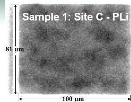
PLI images of small test pads show process induced residual defectivity after USJ implantation and laser thermal annealing
