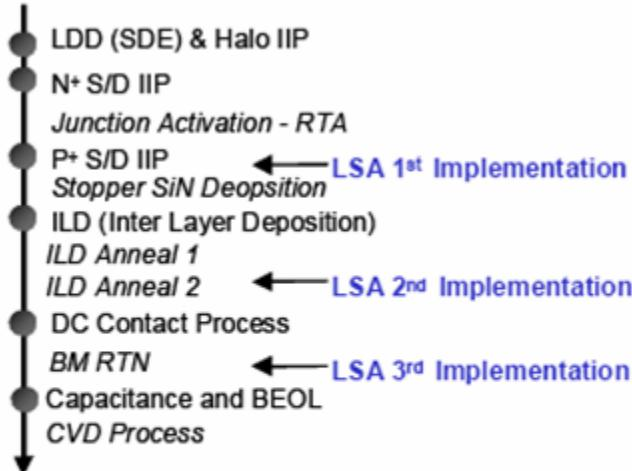
Fig. 1. Process flow after source/drain formation. Some thermal processes at 700 to 900 °C after source/drain activation can cause dopant deactivation.
