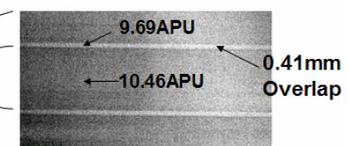
Micro-map showing close-up of striping caused by overlap region
