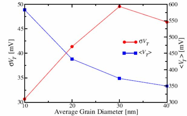
Fig. 3. Dependence of the average threshold voltage,  $\langle V_T \rangle$ , and the standard deviation of the threshold voltage,  $\sigma V_T$ , on the average diameter of the polysilicon grains in a  $30 \times 30$  nm MOSFET assuming midgap Fermi level pinning.
