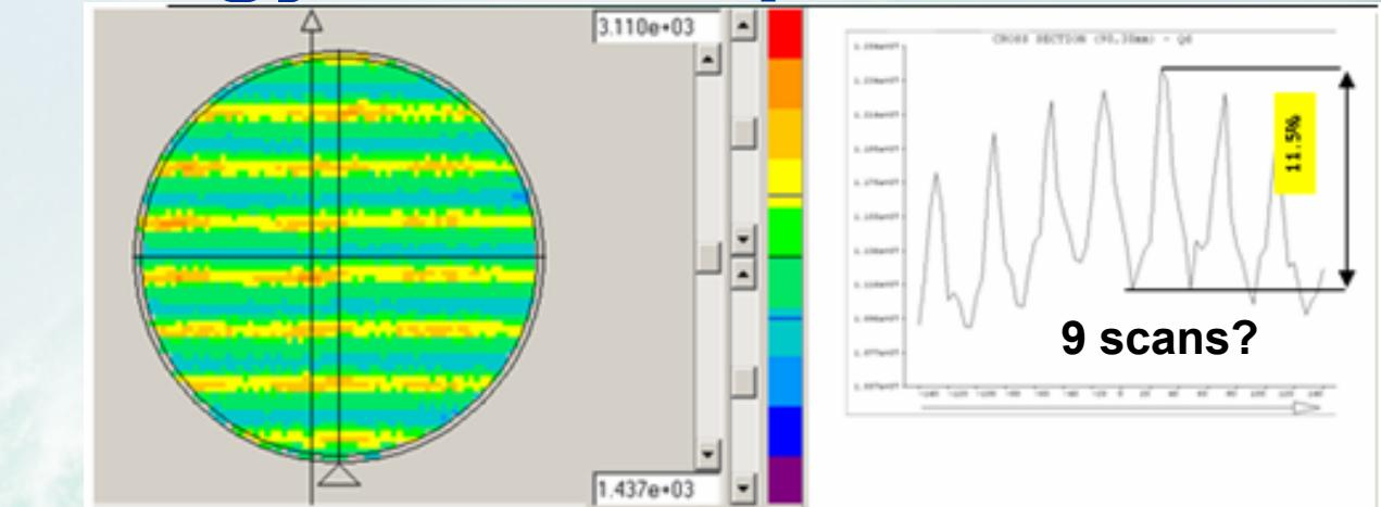
Figure 4a: medium resolution map of a high dose implant from an implanter with two mechanical scans
