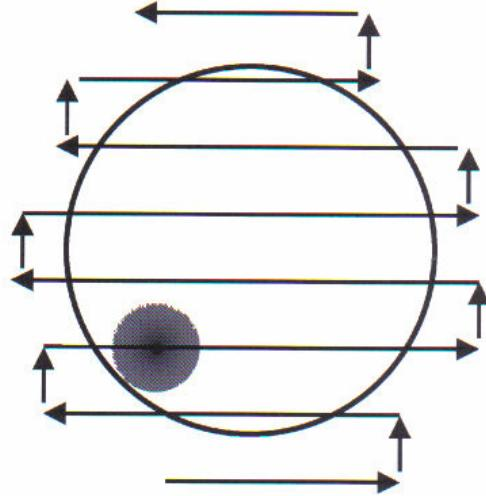
Fig. 4. Double mechanical scan implanter. Schematic showing the locus of the beam centroid in the wafer's frame of reference. The faster mechanical scan axis is horizontal. The wafer vertical position is incremented at the end of each horizontal scan.
