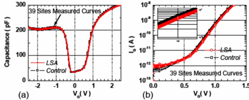
Fig. 15. (a) C-Vcharacteristics for p-FET show no electrical change (EOT) by the LSA in W-gated stack. (b) Gate leakage characteristics show reduction with the additional LSA.
