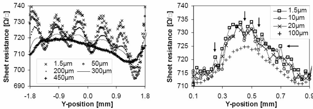
Figure 5: Selected probe pitch and line segment of the 5 mm line scan in figure 3. A line segment was chosen to represent the two main periodic variations of 3.65 mm (left) and ~750  $\mu\text{m}$  (right).
