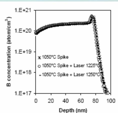
Boron SIMS-profiles in poly-Si with different laser annealing
