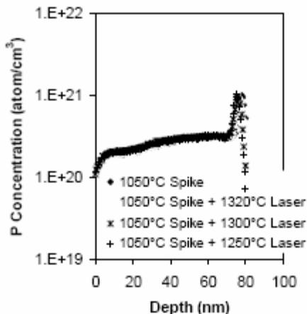
Phosphorus SIMS-profiles in poly-Si with different laser annealing temperatures.
