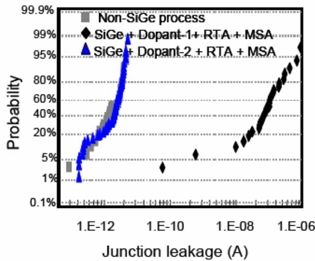
Fig.11 Improved junction leakage due to implant species after MSA.
