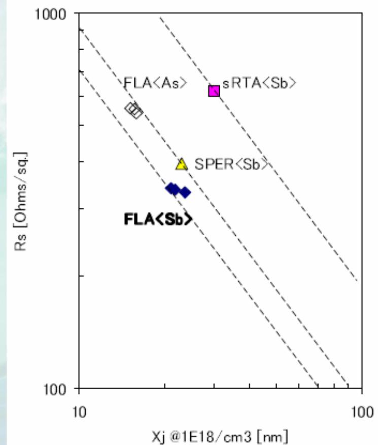
Fig.15 Rs-Xj characteristics annealed by FLA, SPER and FLA (Sb)
