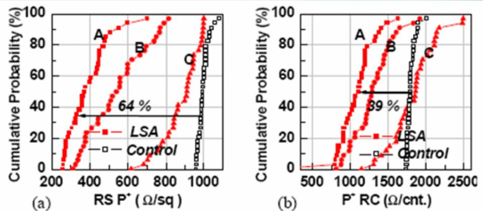
Fig. 3. (a)  $P^+$ /N sheet resistance and (b) contact resistance of peripheral P-FET. Laser annealing was performed with different laser power density (A > B > C) at 3<sup>rd</sup> implementation (reactivation).
