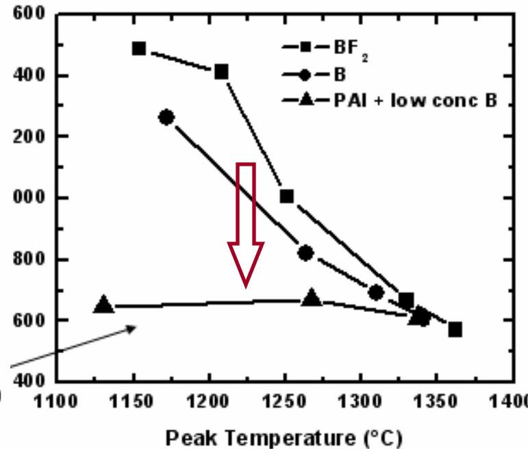
Fig.1 The dependence of lamp power in FLA on Rs of B doped P+/n junction
