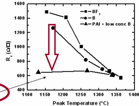
Effect of peak flash temperature on donor activation. There is a significant drop in R<sub>s</sub> with increased peak temperature for non-PAI samples. In comparison, R<sub>s</sub> for the low concentration PAI sample stays level in the temperature range investigated, indicating most of boron is active by 1150°C. (Ref. Mokhberi, Et. Al., IEDM 2002)
