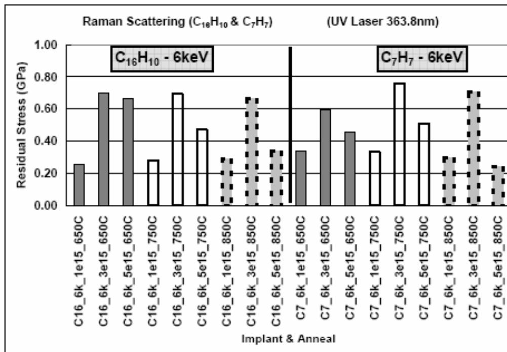
Fig. 10. Stress data for various carbon cluster implant conditions and anneal conditions. Both  $C_{16}$  and  $C_7$  implants are shown to produce similar levels of stress. Data by UV Raman spectroscopy.
