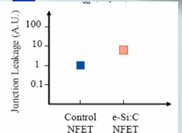
Fig. 10 NFET junction leakage comparison between e-Si:C and control devices. There is a slight leakage increase due to e-Si:C but it is within the acceptable range.
