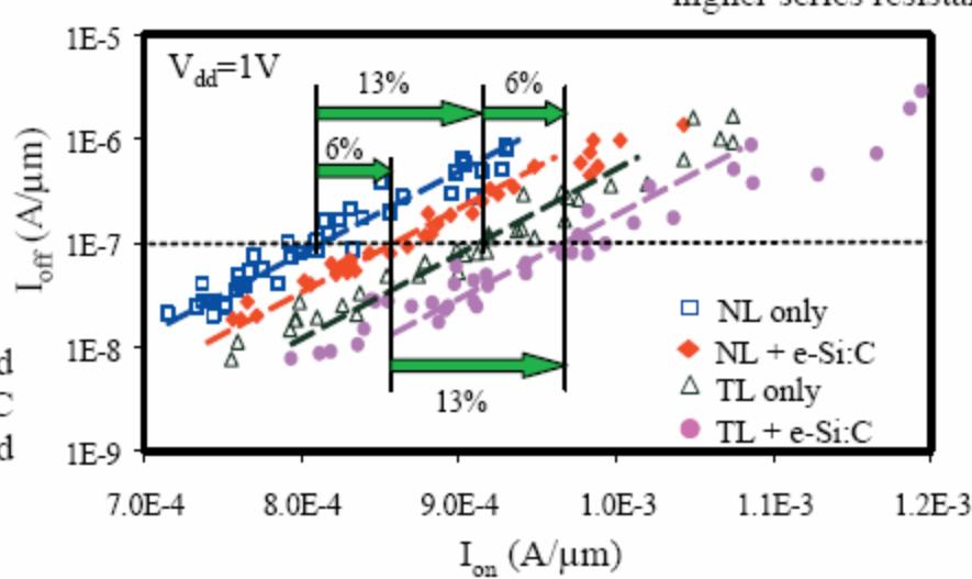
Fig. 8  $I_{on}$ - $I_{off}$  performance comparison for NFETs with different stress elements (NL: neutral liner, TL: tensile liner). Drive current is improved by 6% due to the e-Si:C tensile stressor. When e-Si:C is integrated with TL, both the improvement by e-Si:C (6%) and the improvement by TL (13%) are retained and they are additive to each other.
