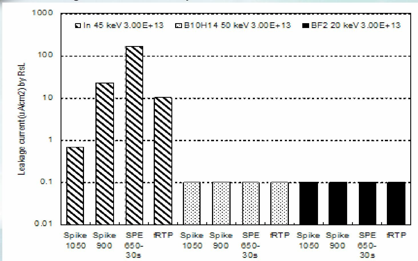
In case of indium I/I, a leakage current was detected by RsL.
