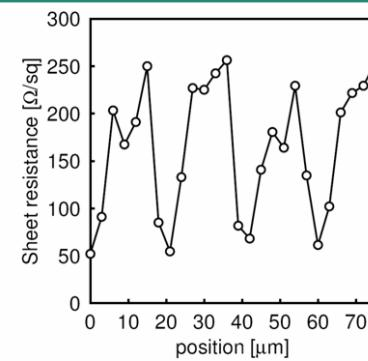
Micro-scale sheet resistance line scan on a Laser Annealed implanted wafer. The probe spacing was 3.0  $\mu\text{m}$ .
