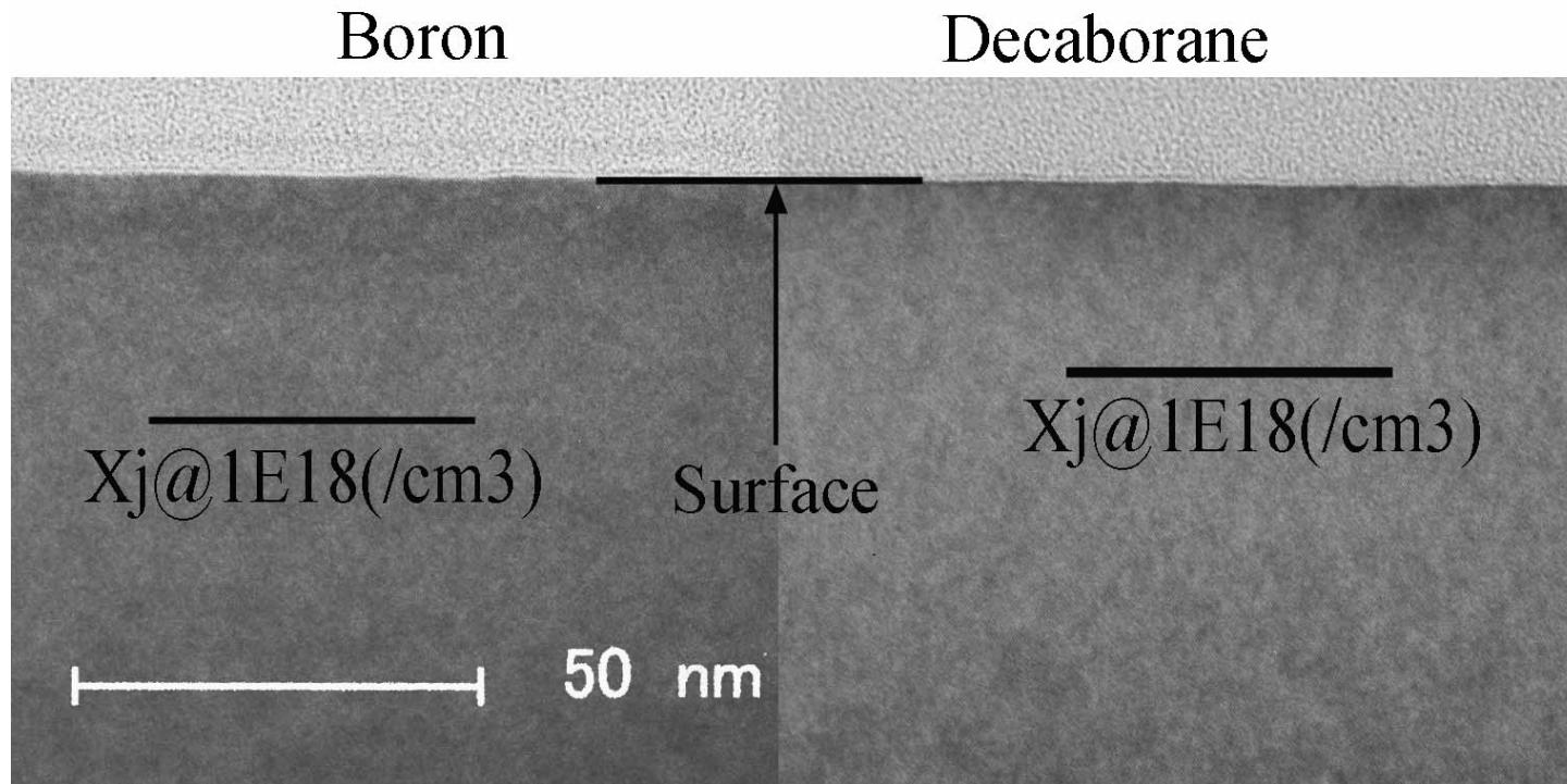
No significant residual defects are observed.
