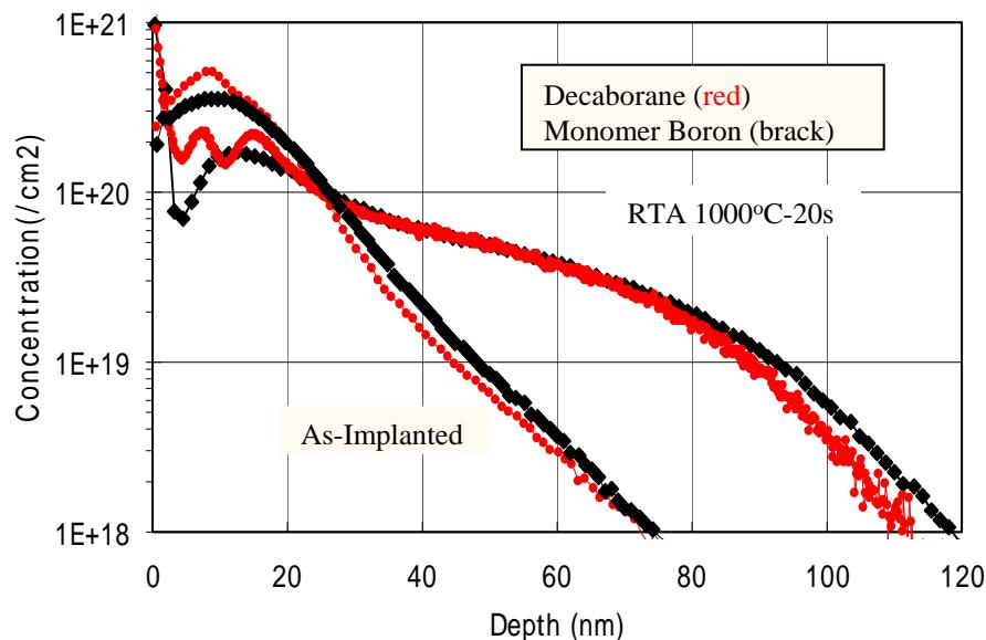
**As-implantation, both profiles are not so much different with  $R_p$  9 - 10nm.**
