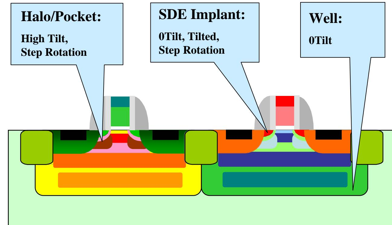
Accurate Dose, Precise Control of Beam Angle & Size
