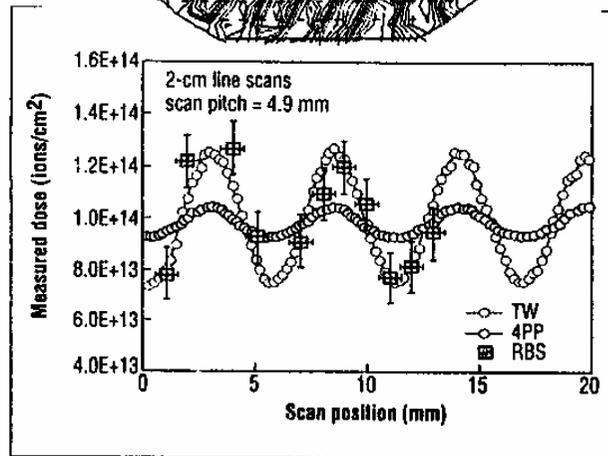
**Figure 7.** Observed dose variations for optical (Therma-Wave), electrical (four-point probe), and physical (RBS) measurements on a wafer implanted with a scan pitch of  $\approx 5$  mm.
