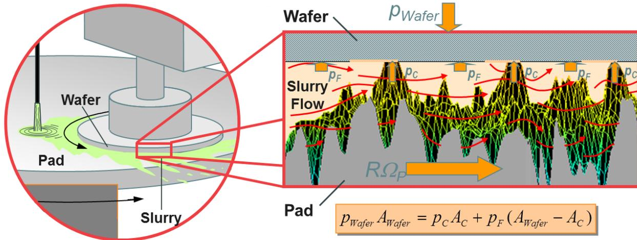
Elevation of wafer above pad is determined by force balances
