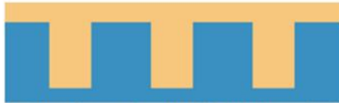
2. Cu planarized with high polish rate
