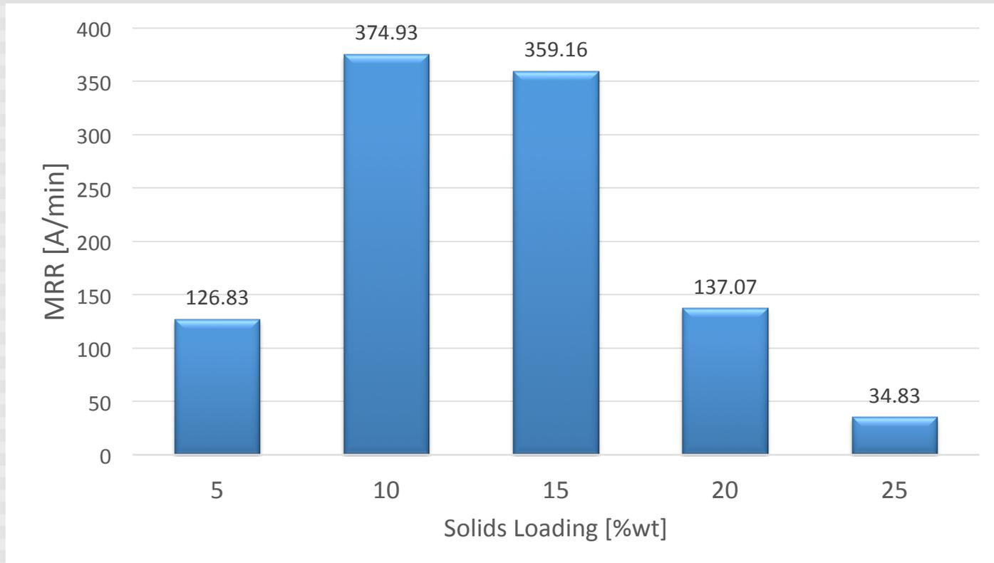
➤ Material removal rate is maximum at 10 wt% solids loading.
