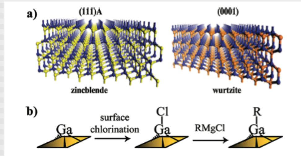
**Figure 1.** (a) Graphical representation of (left) zincblende GaAs and (right) wurtzite GaN crystal slabs. The (111)A and (0001) faces are at the top of each slab, respectively, and feature an atop Ga atom with one bonding orbital not participating in lattice bonding. (b) Wet chemical functionalization of atop Ga atoms at GaAs(111)A and GaN(0001) surfaces through surface Ga–C bonds produced through sequential chlorination and reaction with a Grignard reagent.
