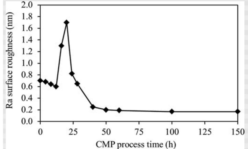
➤ Ra surface roughness measured in  $5 \times 5 \mu\text{m}^2$  plotted as a function of CMP process time.
