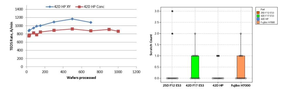
High porosity pads lead to high rate and lower defects
