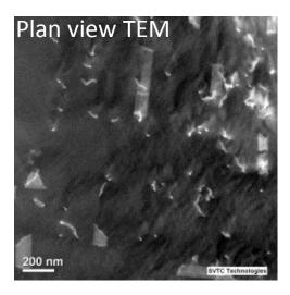
Defectivity ~e9 cm<sup>-2</sup> 'mechanical' wafers for CMP study
