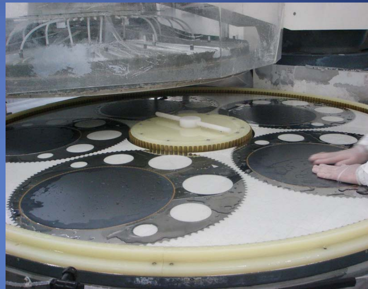
Single Wafer Carrier on Tools for DSP of 450mm Wafers
