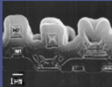
1000 nm Two Al Metal layers, BPSG
