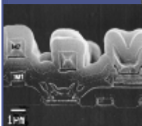
1000 nm Two Al Metal layers, BPSG
