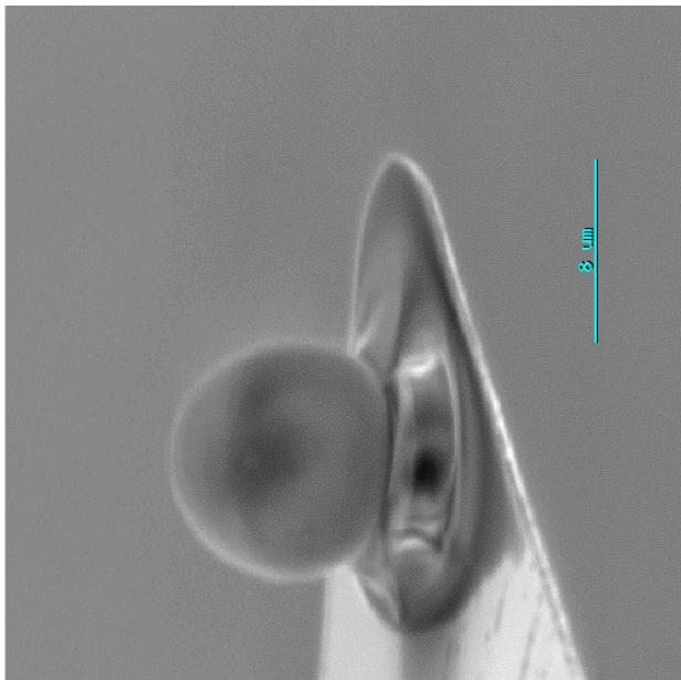
8 micron Silica Particle on an AFM cantilever
