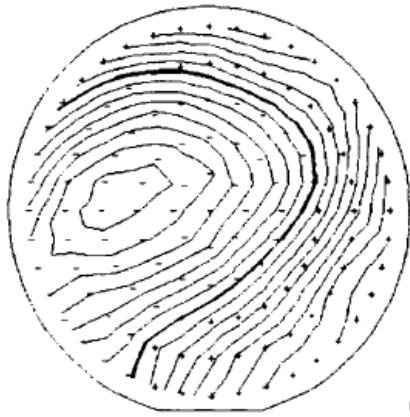
Figure 2. Sheet resistance contour map for axial channeling of 80 keV B ions in a 100mm Si(100) wafer implanted on a mechanical scanned disk with 0° tilt and a center to edge wafer flex of \approx 2^\circ . The ion dose was 7 \times 10^{13} B/cm 2 and the contour intervals above and below the R_{\text{sheet}} average (dark line) is 1% [4].
