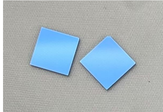
Untreated samples debonded with little force
