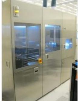
Manufacturer: DISCO Model: DFD 6860 Category: SCRIBING / DICING Vintage: 2015 Wafer Size: 12" Equipment Details: Dicing saw, 12" 2015 vintage.
