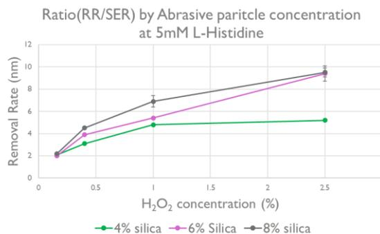
Figure 3 Mo Ratio (RR/SER) results, the effect of H<sub>2</sub>O<sub>2</sub> concentration
