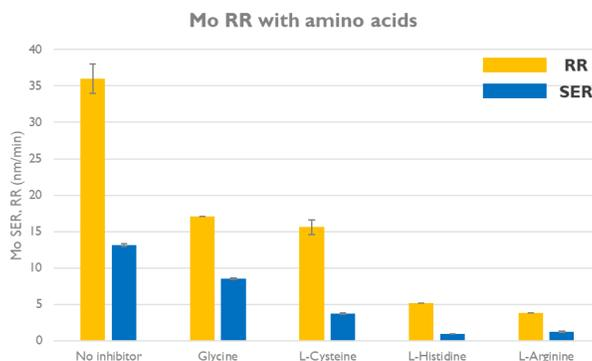
Figure 1 Mo Removal Rate & Static Etch Rate with amino acids
