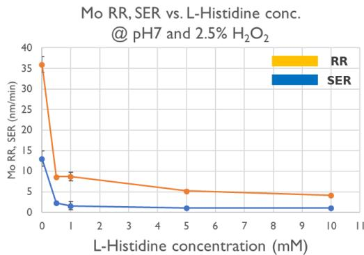
Figure 2 Mo Removal Rate & Static Etch Rate each L-Histidine concentration
