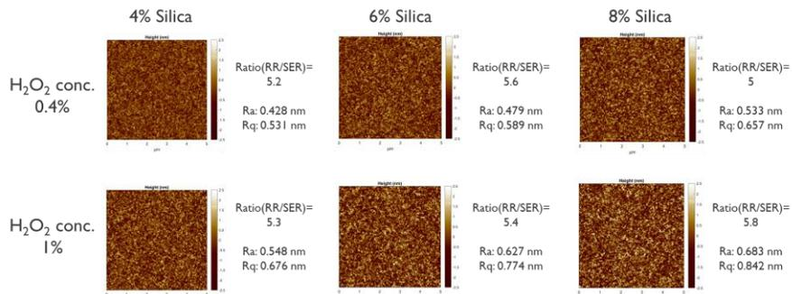
Figure 4 AFM image, Mo surface by silica and H<sub>2</sub>O<sub>2</sub> concentration
