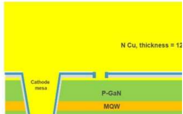
Fig.1 Thick Cu integration for GaN \mu LED
