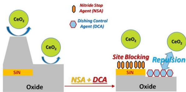
Fig.3 STI slurry design and working mechanism (dual additives system)
