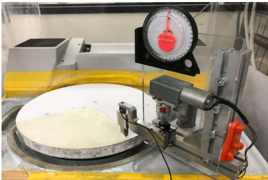
Fig.1 Experiment set up for single-diamond point dressing on PM5 machine.
