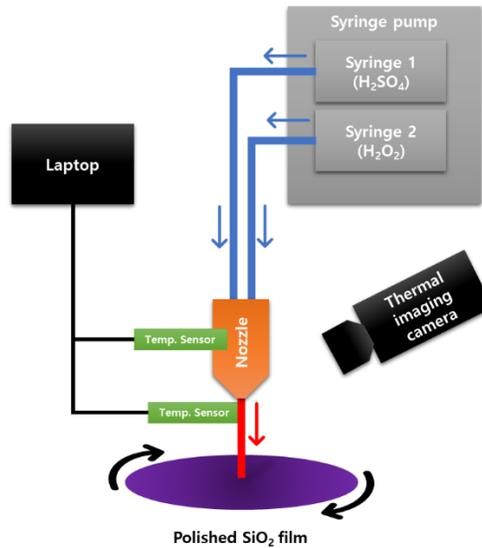
Fig.1 Experimental set-up for verifying expectation of sulfuric acid and hydrogen peroxide reactions and cleaning efficiencies for ceria nanoparticles on the polished SiO<sub>2</sub>
