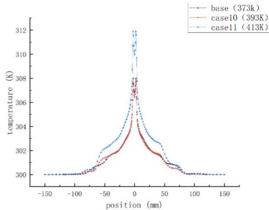
Fig.3 Temperature distributions of SPM solution according to temperature 373 K (black), 393 K (red), and 413 K (blue), respectively
