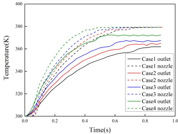
Fig.2 Average temperature development at outlet and in whole SPM spray nozzle
