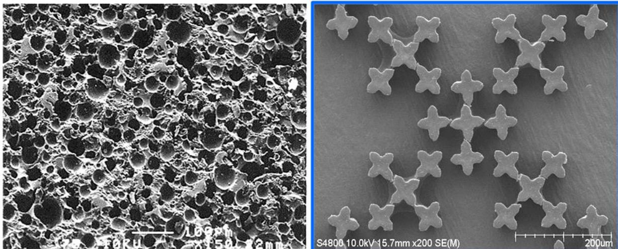
Figure 1: Conventional polishing pad surface (left) and SMART Pad surface (right)
