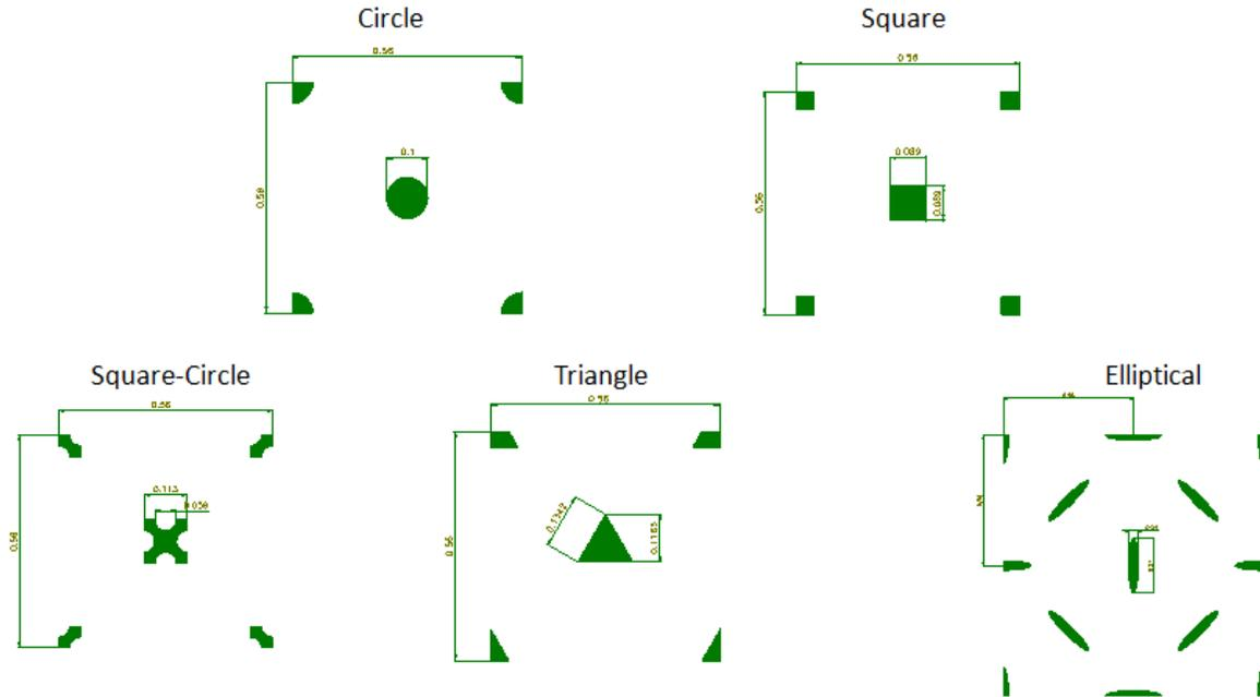
Figure 4: Example micro-feature patterns for the different shapes used in the designs
