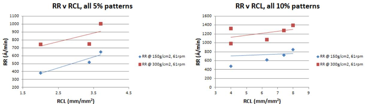
Figure 7: Removal rate versus Real Contact Area for all 5% RCA patterns (left) and all 10% RCA patterns (right)
