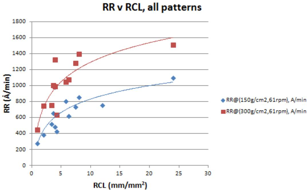
Figure 8: Removal Rate vs Real Contact Length for all patterns
