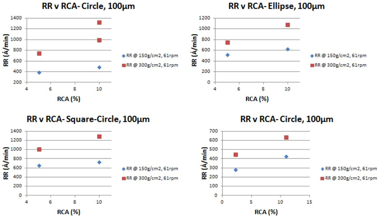
Figure 6: Removal Rate vs Real Contact Area for different micro-feature patterns
