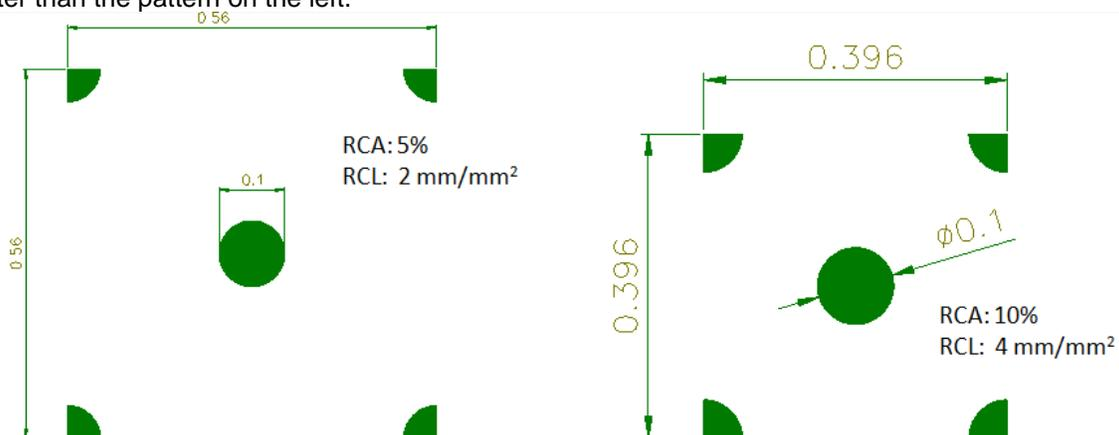
Figure 3: Different values of RCA and RCL for same feature size
