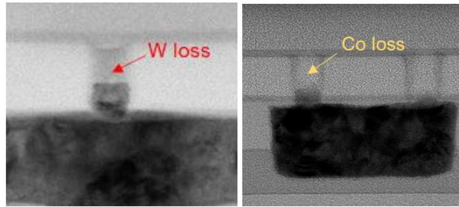
Fig. 8: Cross sectional TEM pictures showing excessive W loss (*left*) and Co loss (*right*) after CMP.
