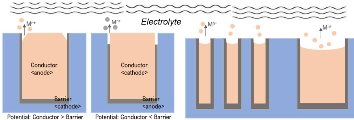
Fig. 1: Cu metal loss due to galvanic corrosion (*left*) and chemical etching (*right*).
