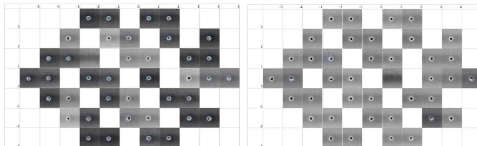
Fig. 3: Top-down SEM inspection on isolated Cu via patterns on 39 dies across a POR wafer (*left*), and a wafer that received 2X longer post polish 5MBTA rinse (*right*).
