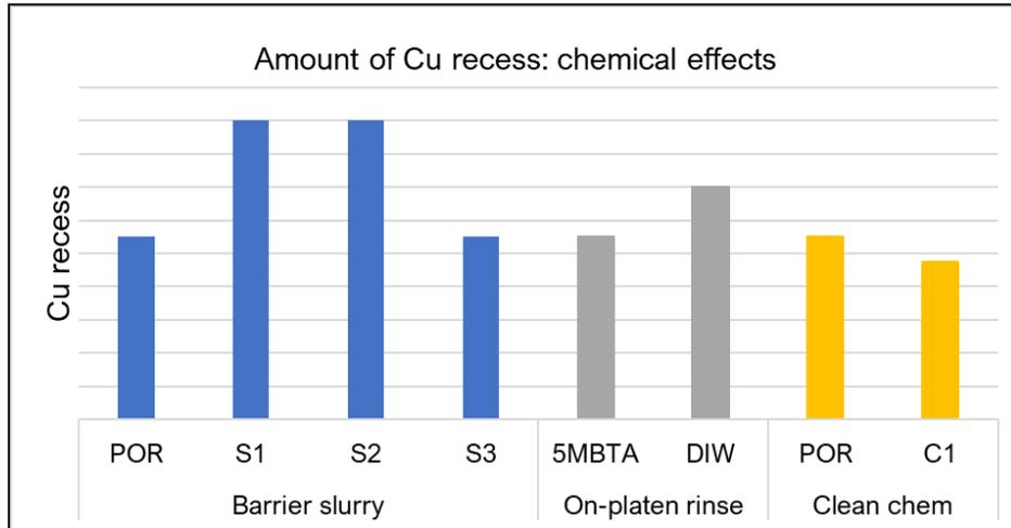
Fig. 4: Effects of barrier slurry, on-platen rinse, and post CMP clean chemical on Cu recess.
