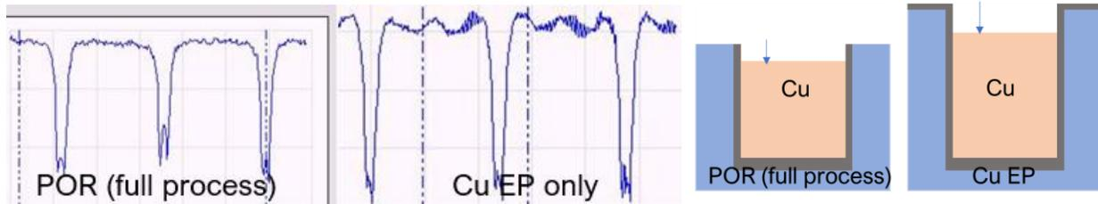
Fig. 6: AFM traces over Cu vias of POR vs Cu EP only wafers (*left*); and illustration of the difference in amount of Cu recess between the 2 wafers. (*right*).
