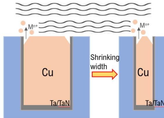
Fig. 7: Metal loss from galvanic corrosion between Cu and Ta/TaN liner.
