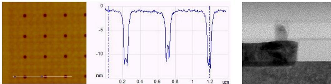
Fig.2: Metal recess in fine Cu vias after CMP as suggested by AFM scan and confirmed by cross-sectional TEM picture.
