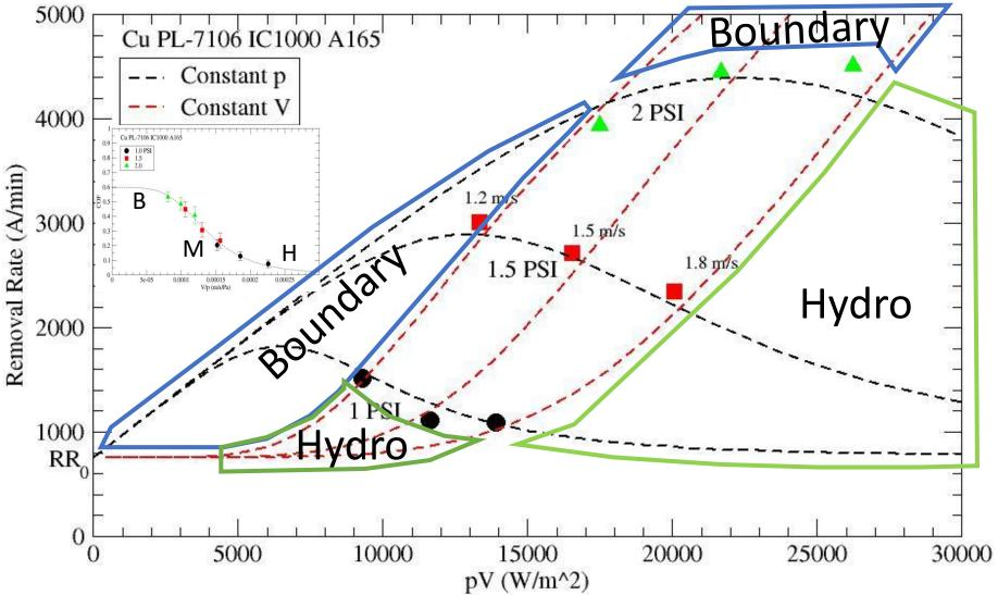
The model predicts a pressure threshold for shear force removal. At the given speeds, this is just the minimum p Needed to overcome summit/wafer)lubrication and begin engaging in solid/solid contact.
