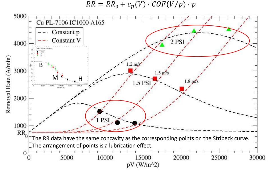
The points in the convex hull of the data all lie in the mixed lubrication part of the Stribeck curve where there is plenty of data. The interpolation in this region is reliable.
