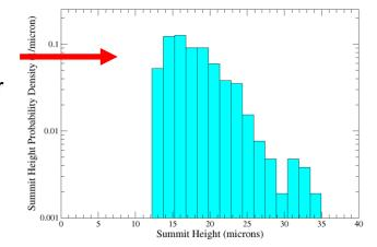
Calculated reaction temperatures are the *mean or expected value* taking into account all contacting summits and their distribution of heights, curvatures, actual contact pressures, and lubrication layer thicknesses.
