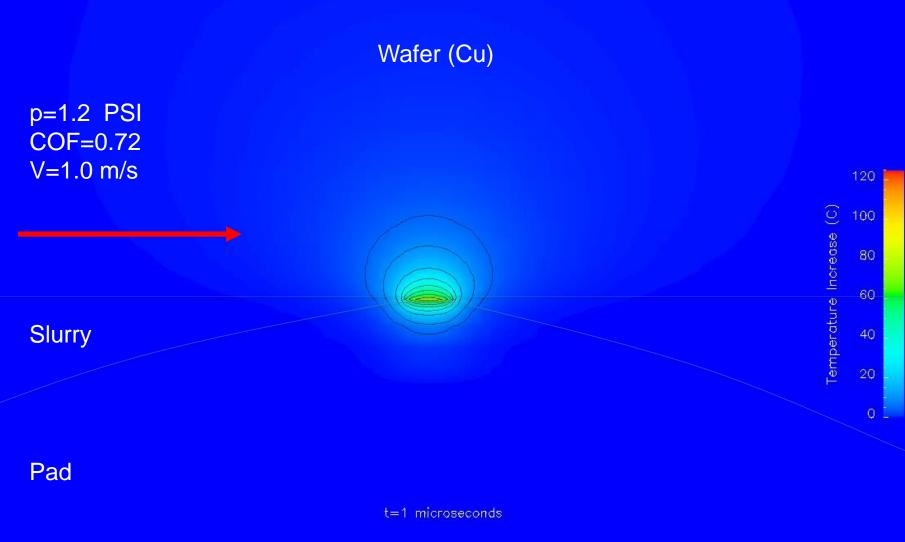
$\Delta T$  reaches steady state very quickly, so it is constant over most of the wafer.
